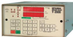
The electronic trip relay can be checked by this field test device when the breaker is at test position or disconnect position. The breaker will trip when tested with this device.
