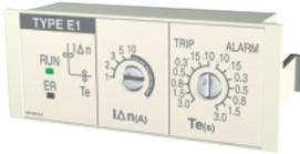
By combining the ETR with earth leakage protection (ER) and External ZCT, earth leakage protection is possible. Earth leakage protection, earth leakage tripping and earth leakage alarm can be selected. Control supply is necessary for this function.
