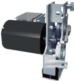
The closing spring is charged by an electric motor. When the breaker is closed, the spring is charged automatically (ON-charge method.) The closing coil (CC) is required to remotely close, and the shunt trip device is required to remotely open the breaker.
