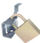
This kit is used to lock the safety shutters using 2 padlocks (the padlocks to be customer's supply). The safety shutters close when the breakers drawn out to prevent accidental contact with the main contacts.
