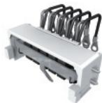
When moving the breaker from the connected to the test positions, this contact is used to short circuit auxiliary switch (AXb) thus maintaining the correct sequence of operation of the external control circuit. When ordering, SBC with the same number of contacts as auxiliary switches (AXb) will be provided.
