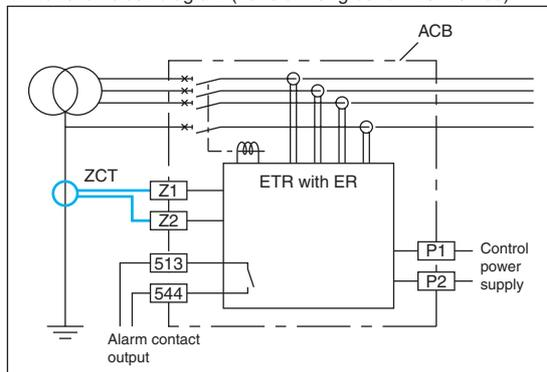
Earth leakage protection characteristics
