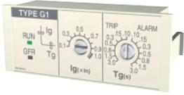
The ground fault protection (GFR) of several hundred amperes is possible. This function can be selected for trip and alarm (no trip). Power supply is necessary for this function, even if there is not power supply, it can function at  $0.2xI_n$  or higher.
