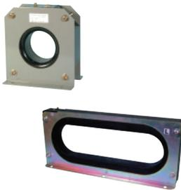
This option is used to detect several amperes of earth leakage when use in combination with a electronic trip relay that has the earth leakage tripping (ER) option. Two methods are available. The first is where the all load conductors pass through the ZCT. The other method uses a smaller ZCT through which the supply transformer's ground wire passes through to earth.
