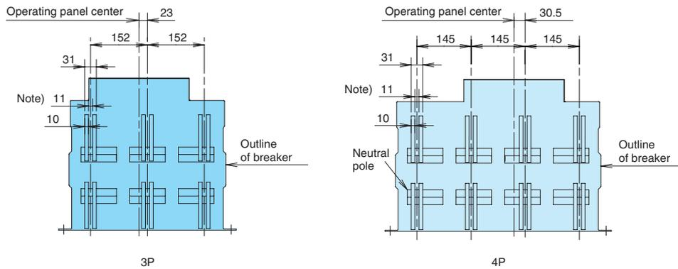
Note) Spacers are not required when fastening connecting conductors (T10). The necessary contact area can be obtained with ACB terminal bent by tightening the screw.
