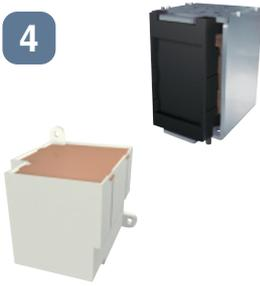
This is the device that automatically trips the breaker when the circuit voltage drops below the nominal voltage, and comprises UVT coil and UVT controller. There are 3 kinds of tripping time, INST, 0.5s and 3.0s.
