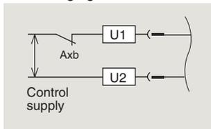
OFF charging method is also available. The closing spring is charged automatically when the breaker is opened. This is available only by externally connecting b contact (AXb) of the auxiliary switch to the motor charging circuit in series. In case of DC power supply, please use high capacity auxiliary switch (HAX).
